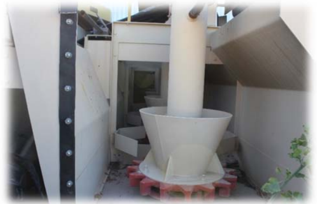
Refurbished Flotation Cell
